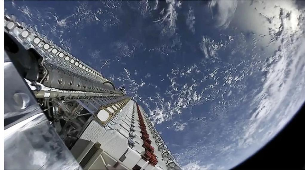
Typical mass launch of Starlink blade satellites with one rocket (60 satellites with Falcon 9, 25.5.2019)
